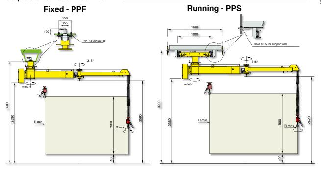
Air supply: Dry and oil-free compressed air min constant 0.7÷0.8 MPa
