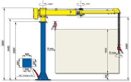
Structural versions: column mounted on fixed base-plate, autostable base-plate of our supply properly dimensioned.
